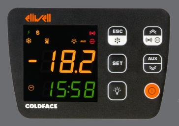
The large LED display allows constant monitoring of cold room status
